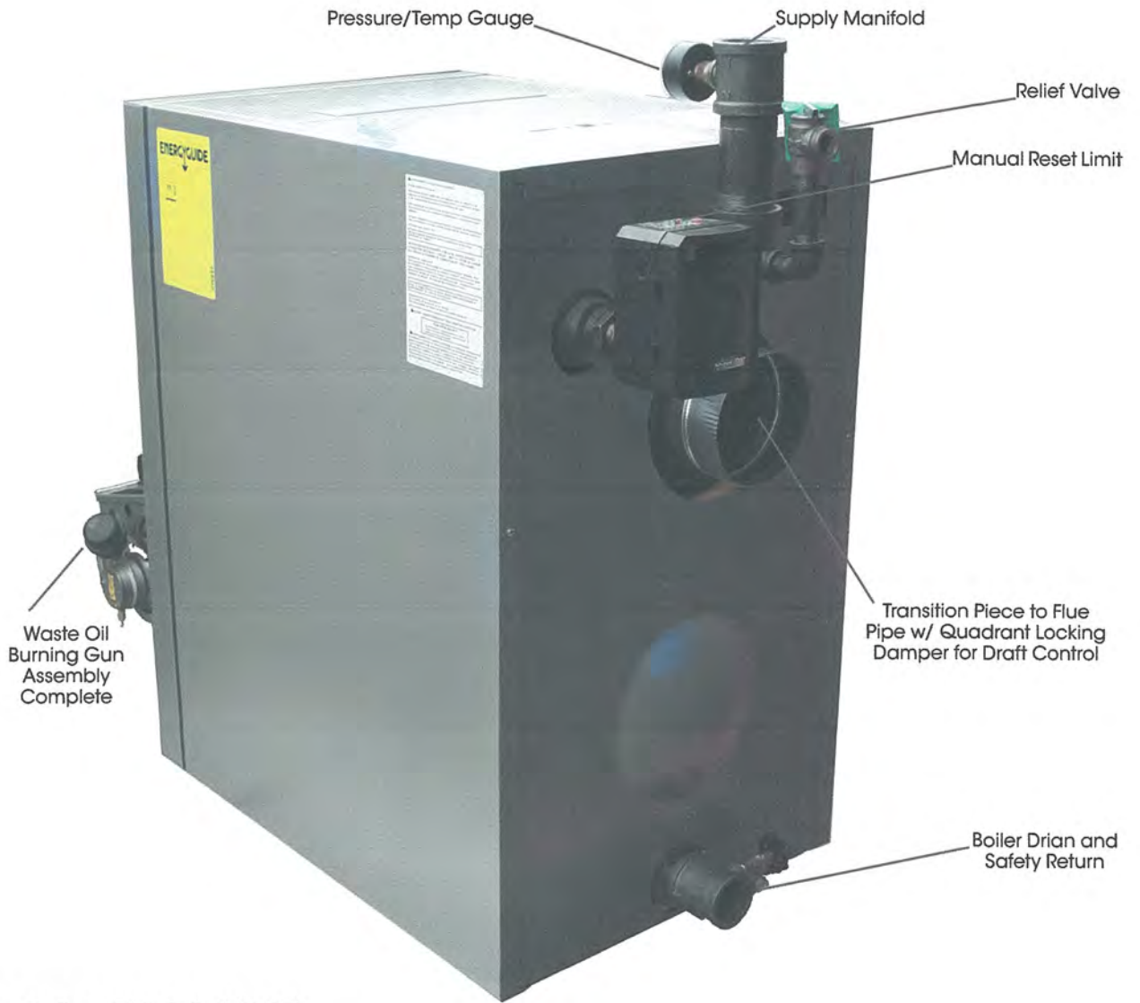
Figure 10 - Boiler (WB-9 & WB-15)
