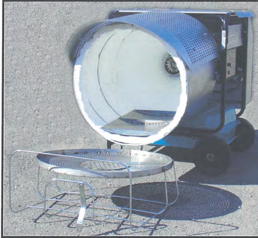
Figure 15 – Combustion Chamber Cleanout Door
