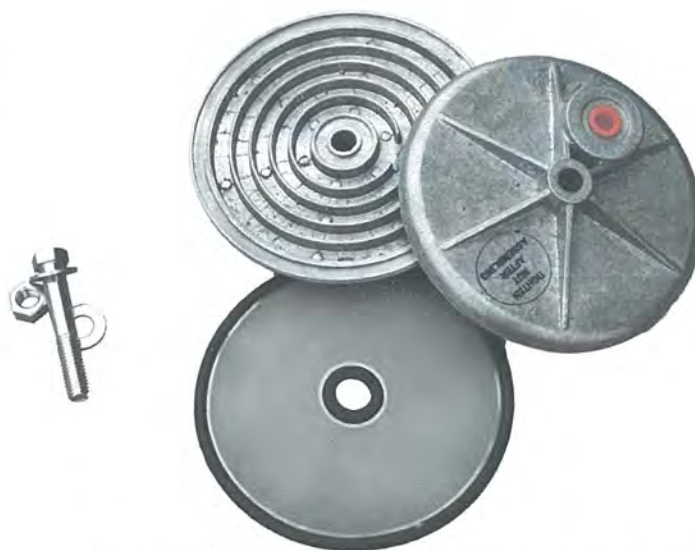
Figure 41 - Oil Filter (Spin-On Filter above, Pancake Style Filter below)
